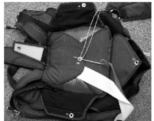
**# 12** Pack one third of the remaining bridle (approx. 3 feet) by making long S-folds in the bridle from top of the bag to the bottom right hand corner as shown. Repeat the process on the left side with the remaining third of the bridle—making the S-folds from top of the bag to the left-hand corner of the container shaping a big V.
