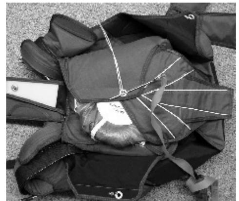
**# 16** Close the left top flap #5 and secure it with the TLP you used on top flap #4.
