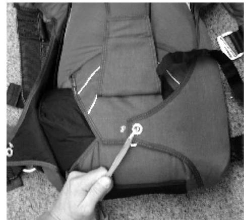
**# 6** and thread the pull-up cord through the #4 flap on the left.
